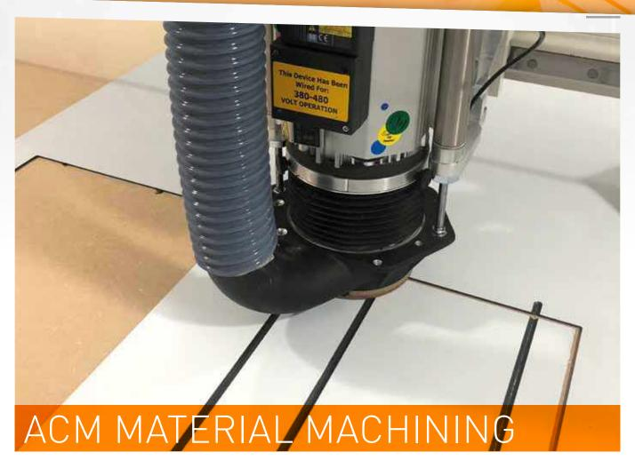
At ITC we understand the constant pressure our customers are under to be price competitive, often involving using less expensive ACM (Aluminium Composite Material) sheet material. This can cause real issues for the customer, as they may find their usual tools aren't lasting as long as they have previously. Sometimes less expensive ACM sheets use recycled substrates in their composition which result in poor surface finish and reduced tool life.
